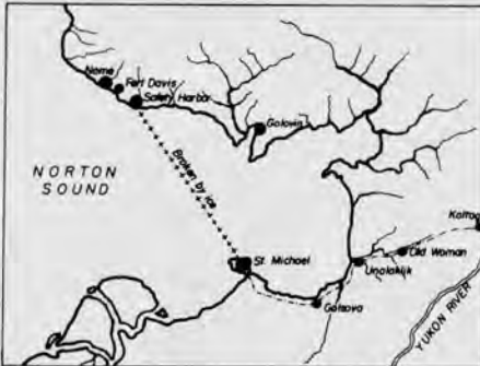
Map showing the wireless circuit between Nome and Fort St. Michael, Alaska, a distance of 100 miles. This circuit was put into operation by the U.S. Signal Corps in 1903 to replace the cable which was washed out by ice every year.
